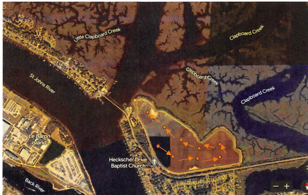
Figure 1. Estimated spoil sample sites. Orange circles represent approximate push core sample sites, orange arrows indicate probable flow path of dredge materials.
