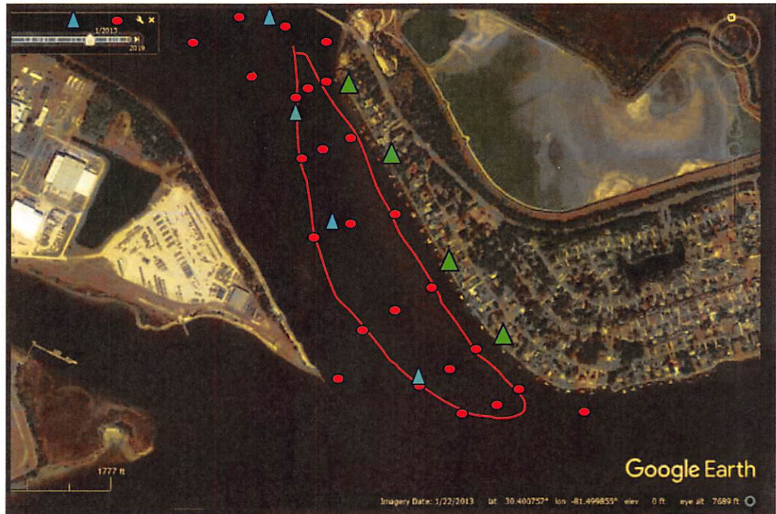
Figure 2. Probable push core locations in river sediments and submarine/subaerial trap locations. The solid red line indicates the approximate outline of the shoal, red circles indicate push core samples, blue triangles subaquatic magnetic traps, and green triangles subaerial filter traps.
